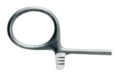
**Step 7: Profile Grinding.** After the forged parts are milled, they are ground on a rough stone grinding wheel. This step removes any excess material that may be remaining after the forging process.
