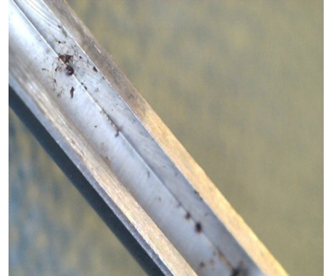
Figure 3: A dirty slide shaft
